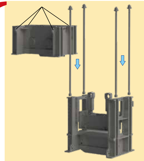
Conventional method: insert tie-rods from above
