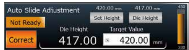
Display of automatic slide adjustment
