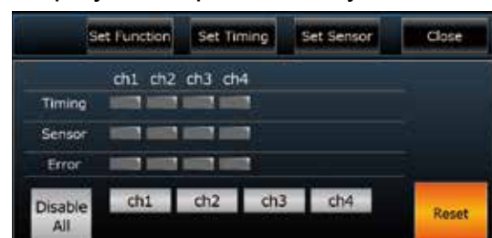
Display of die protection system
