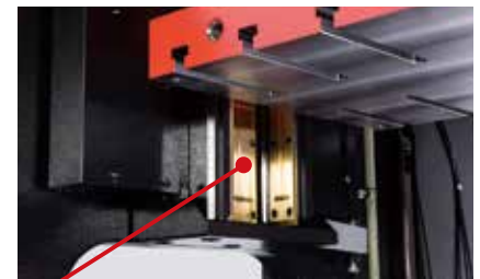
Center-gib full-guide structure
