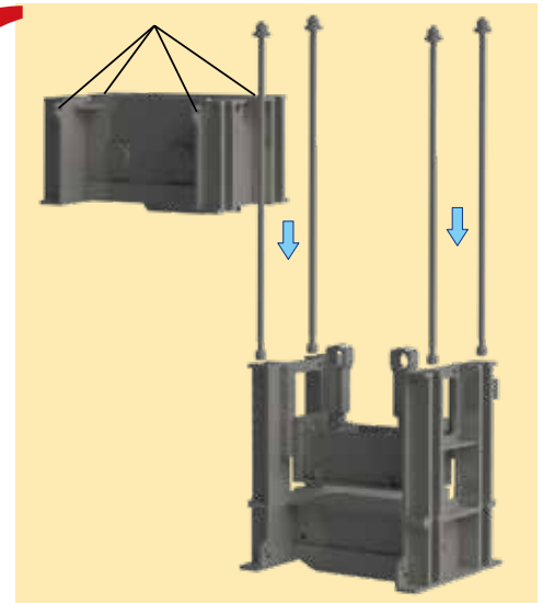
Conventional method: insert tie-rods from above
